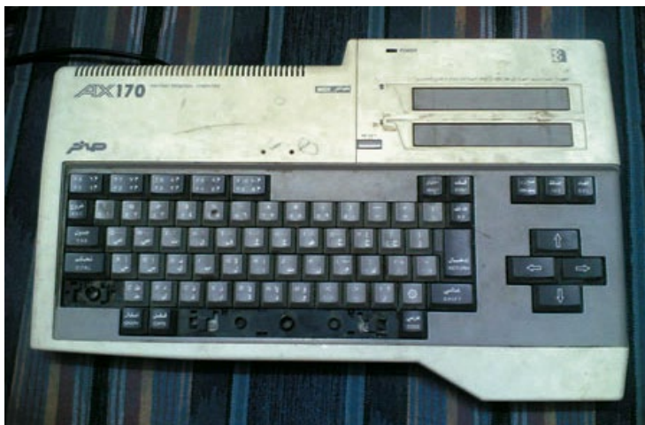
During the 1980s, many budding Arab developers got started with the Sakhr line of microcomputers, based on various iterations of the MSX format, with Arabic software. "It defined our generation," Samer Abbas says
